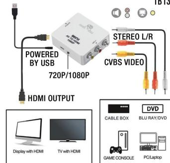
It converts RCA (AV, composite, CVBS) signals into HDMI signals so you can watch your video on a modern TV with HDMI port. The analog to digital conversion in this module employs 10 bits maximal 162MSPS sampling, black/white level expansion, color transition improvement, dynamic range expansion, blue stretch, auto-detect and auto-convert the composite signal to 1080p(60HZ) output. Making video come alive, delivering the sharpest, most realistic HD visuals available.
