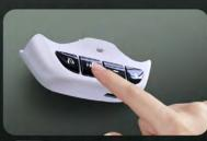
Press and hold the paring button for 3s to turn on, Red and blue lights flash alternately.
